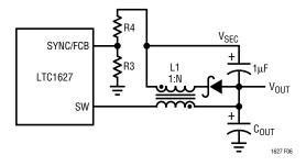
Figure 6. Secondary Output Loop Connection
