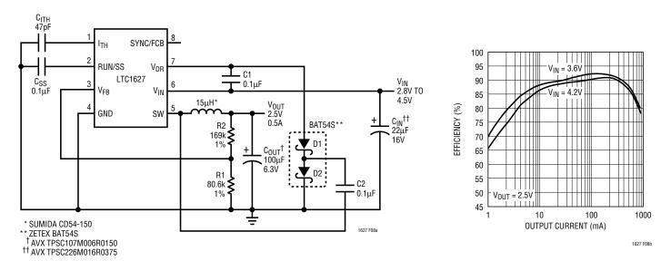
Figure 8. Single Lithium-Ion to 2.5V/0.5A Regulator
