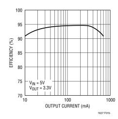
Figure 1b. Efficiency vs Output Load Current
