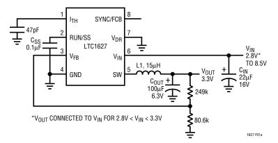
Figure 1a. High Efficiency Step-Down Converter
