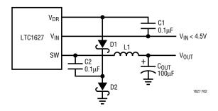
Figure 2. Using a Charge Pump to Bias  $V_{DR}$
