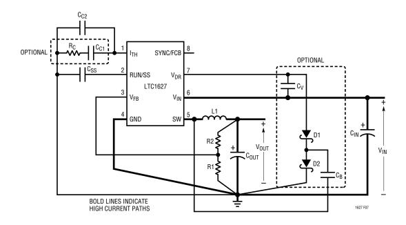
Figure 7. LTC1627 Layout Diagram
