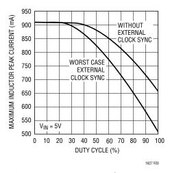
Figure 3. Maximum Inductor Peak Current vs Duty Cycle
