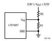
Figure 4. Setting the LTC1627 Output Voltage
